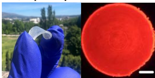
Fig. 1. Physical appearance of AC/IS-EuTbEr monolith under daylight (left) and UV radiation (365 nm) (right). The scale bar is 1.0 cm.
